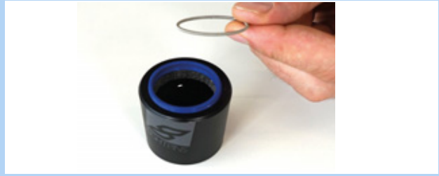
Figure 172: Removed spring washer
