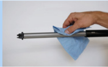
Figure 216: Cleaning the longitudinal groove
