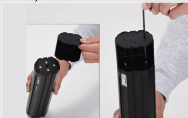
Figure 32: Fitting the PowerTube extension
