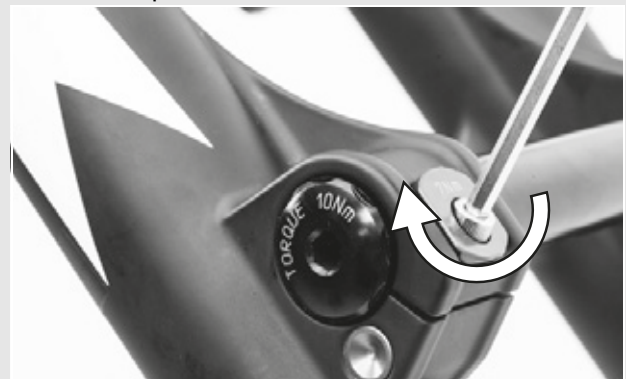
Figure 40: Tightening the securing clip
