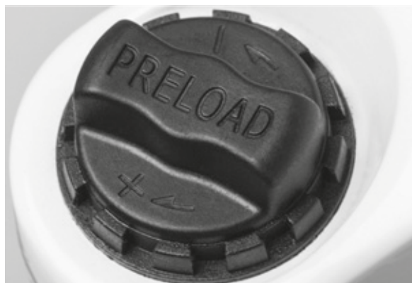
Figure 64: Negative deflection setting wheel on the suspension fork crown
