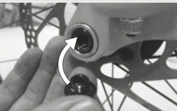
Figure 37: Pushing the quick release lever into the axle
