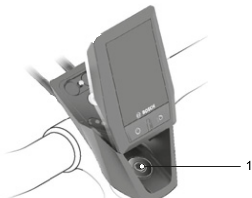
Figure 72: Position of headset screw
