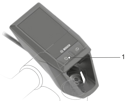
Figure 74: Position of On-Off button (on-board computer)
