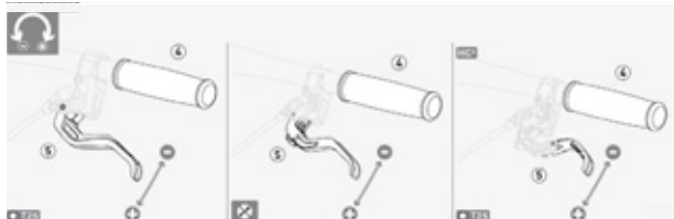
Figure 62: Setting the grip distance on a Magura disc brake lever
