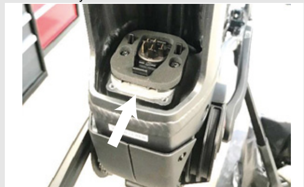
Figure 26: Fitted adapter plates
