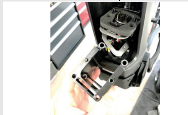
Figure 25: Pulling out the PowerTube adapter
