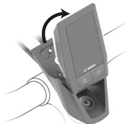
Figure 73: Removing the on-board computer.
