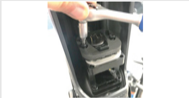
Figure 22: Undoing screws on battery mount
