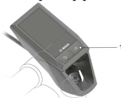
Figure 75: Position of riding light button
