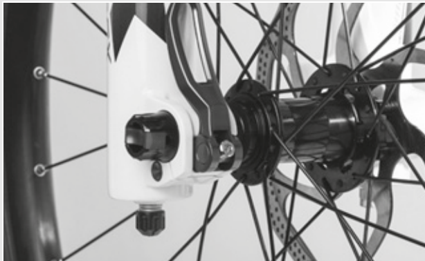
Figure 45: Perfect position for the clamping lever
