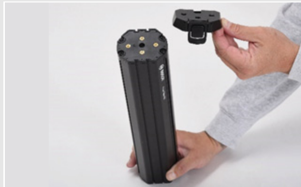
Figure 29: Fitting the mounting plate
