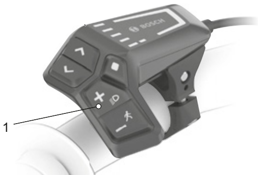
Figure 105: Position of riding light button (1)
