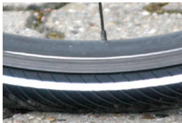
Figure 78: Correct tyre pressure. The tyre is barely deformed under the load of the body weight
