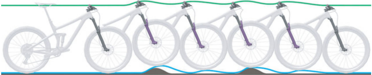
Figure 196: Suspension fork rebounding too quickly
