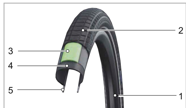
Figure 21: Structure of tube-type tyre
