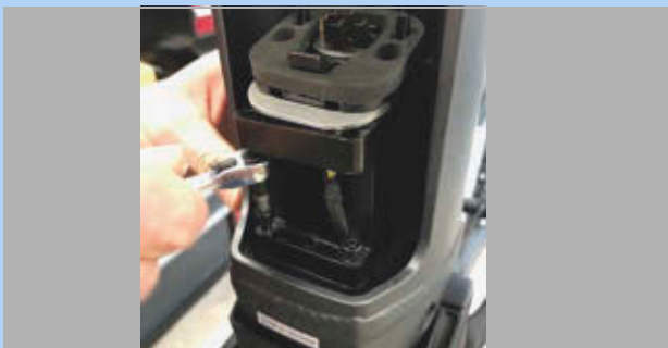
Figure 71: Removing the 4 mm hexagon screws
