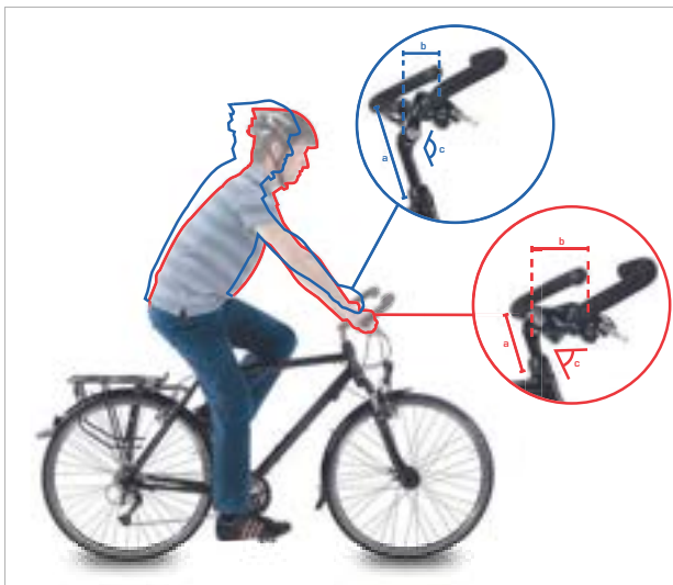
Figure 125: City bike (blue) and trekking bike position (red) by changing the angle
