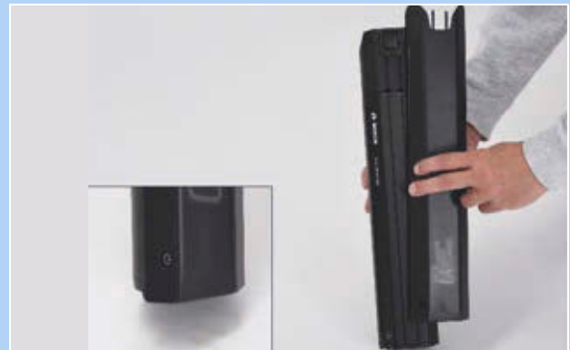
Figure 82: Pushing the battery cover onto battery
