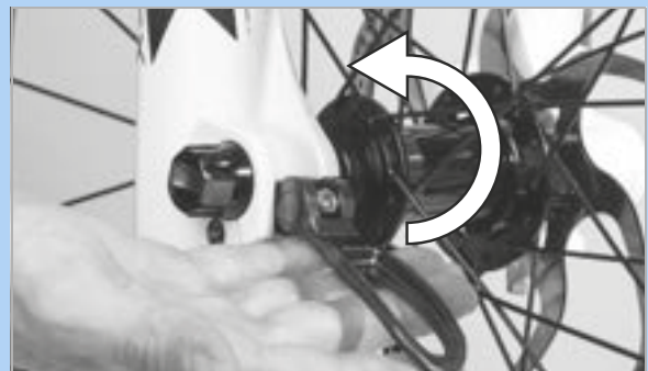
Figure 93: Pressing the quick release lever in the direction of the arrow
