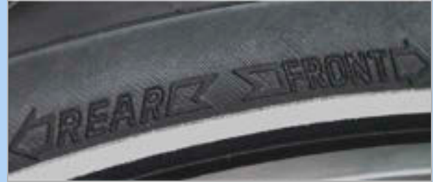
Figure 85: Rotation direction arrow on MTB tyres
