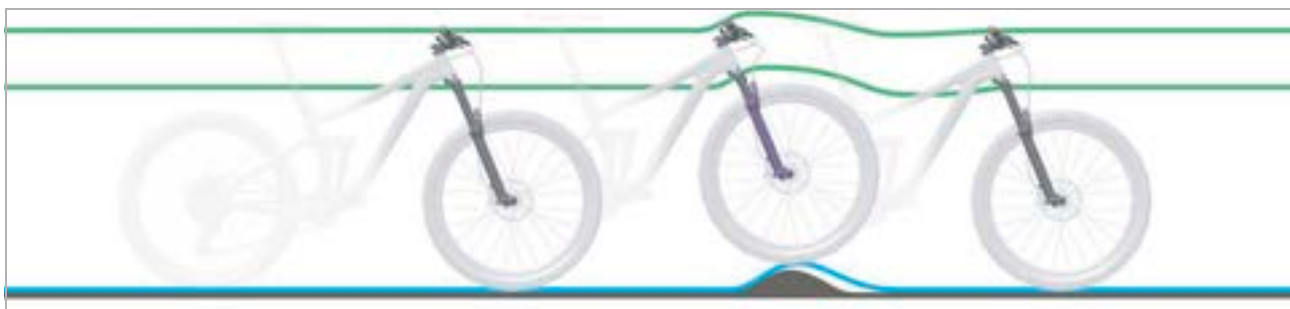
Figure 196: Excessively hard damping in the suspension fork on bumps
