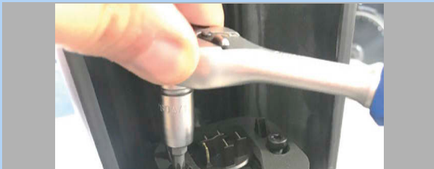
Figure 70: Undoing screws on battery mount
