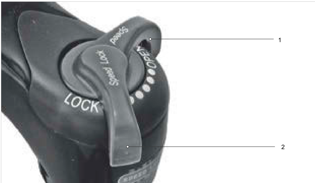
Figure 165: SR SUNTOUR compression adjuster in open (1) and closed (2) position
