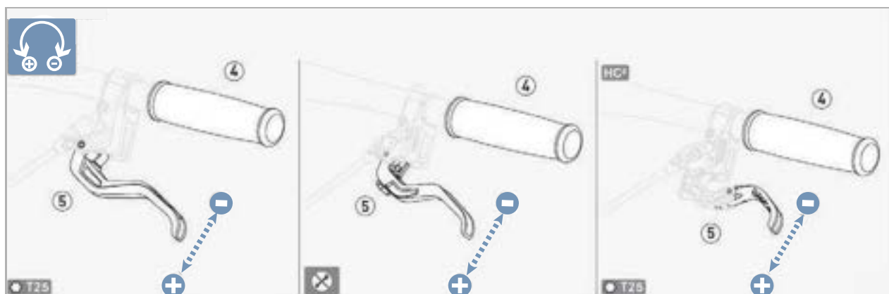
Figure 133: Adjusting the grip distance for a MAGURA handbrake disc brake
