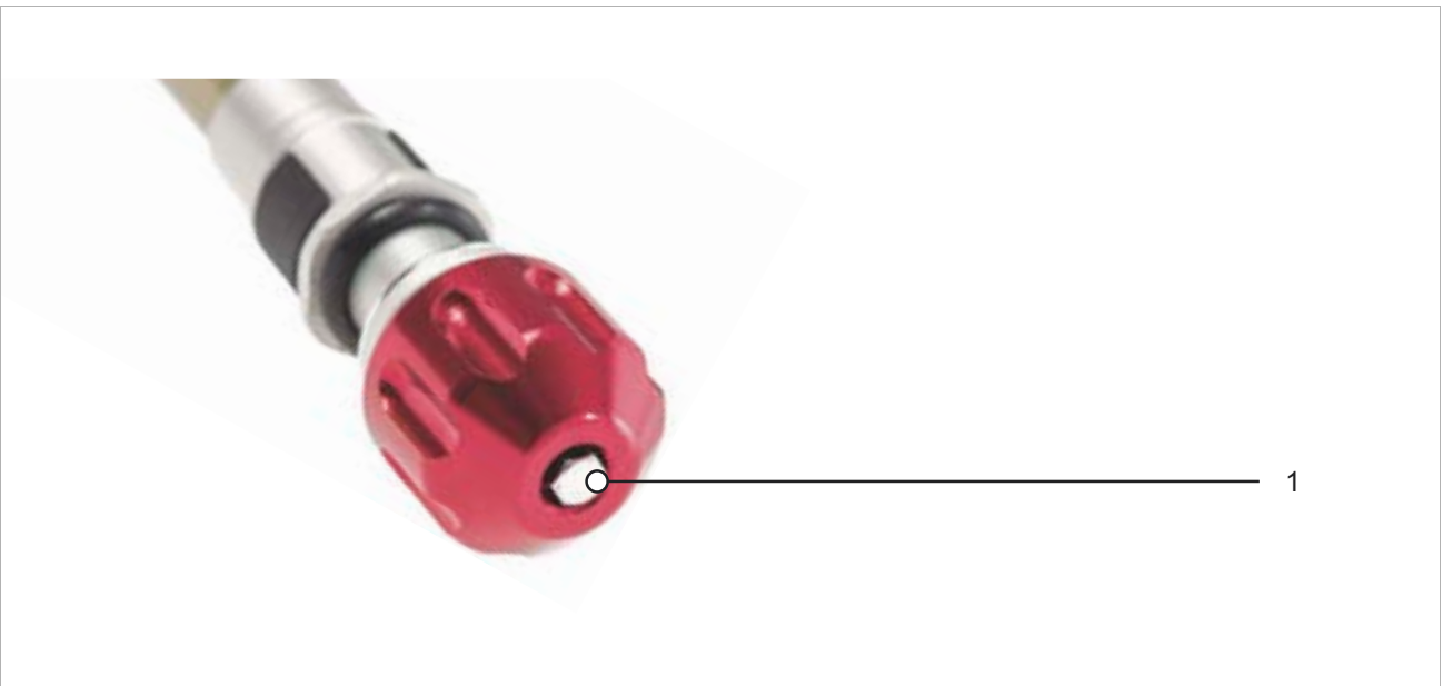
Figure 194: Example of SR SUNTOUR rebound screw (1)
