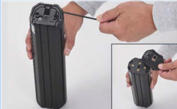
Figure 76: Detaching the upper interface
