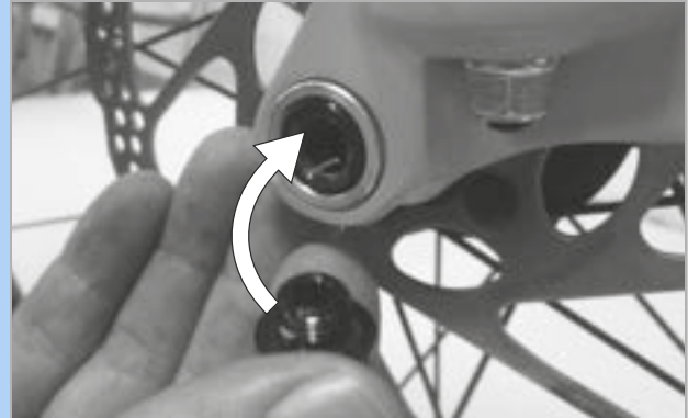
Figure 88: Inserting the securing screw
