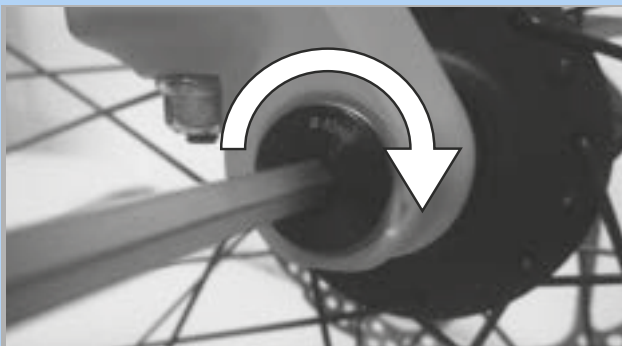
Figure 87: Tighten the axle in the direction of the arrow
