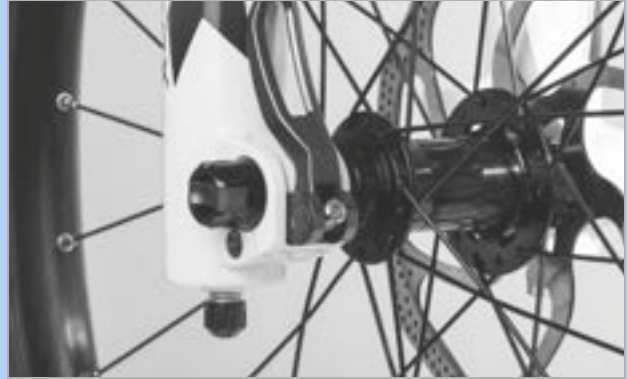
Figure 187: Adjusting the quick release clamping force
