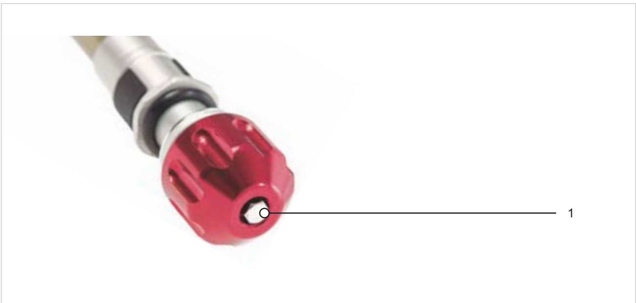
Figure 192: Example of SR SUNTOUR rebound screw (1)
