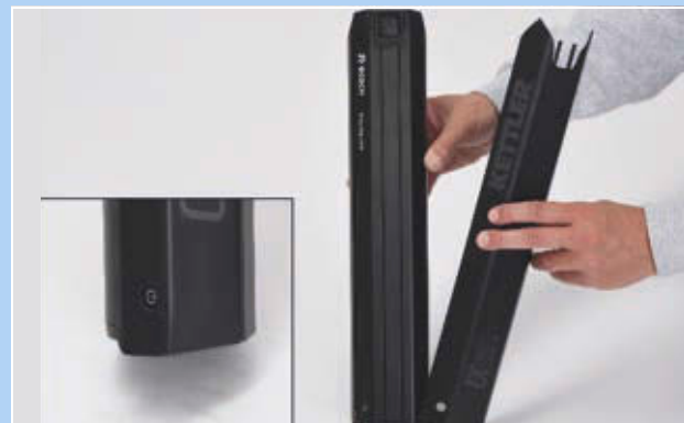
Figure 78: Pushing the battery cover onto battery
