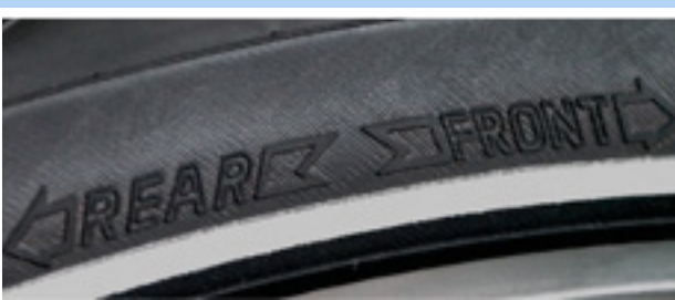
Figure 50: Rotation direction arrow on MTB tyres
