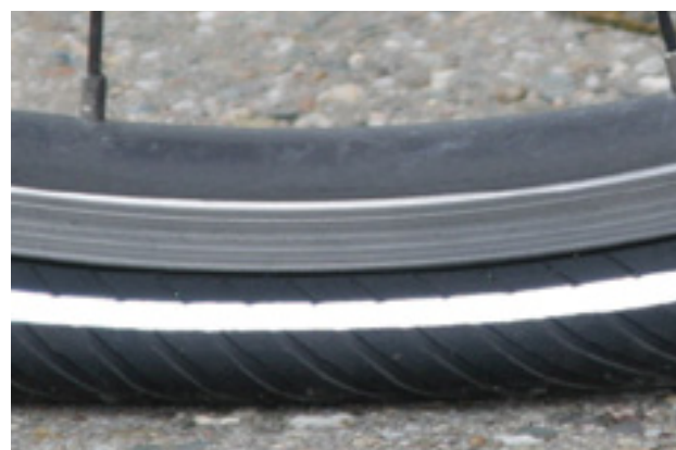
Figure 87: Much too little tyre pressure
