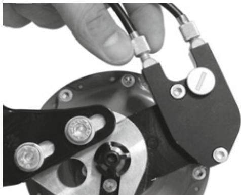
Figure 135: The tension adjuster on Rohloff hub versions with external switch control is located on the cable box positioned on the left-hand side
