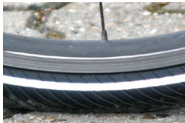
Figure 86: Correct tyre pressure. The tyre is barely deformed under the load of the body weight
