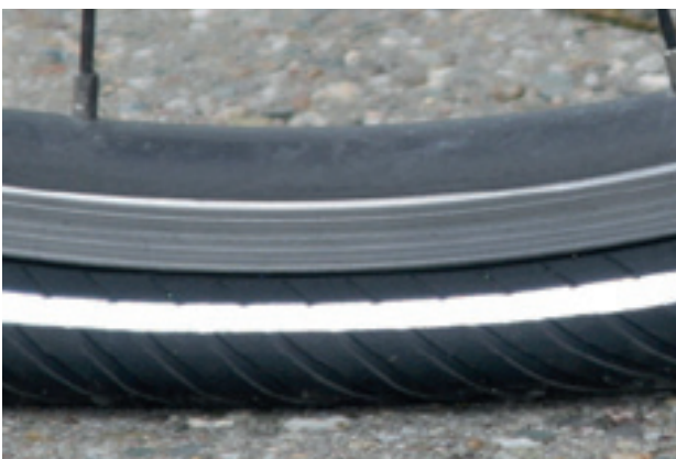
Illustration 97 : Pression largement insuffisante
