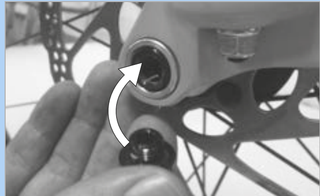
Figure 86: Inserting the securing screw
