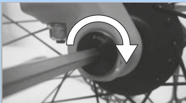
Figure 85: Tighten the axle in the direction of the arrow
