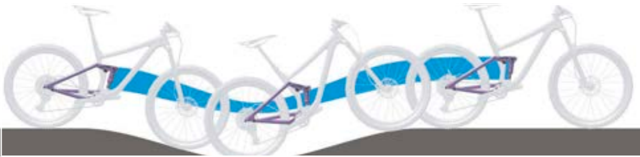
Figure 238: Excessively soft suspension in the rear frame damper on hilly terrain
