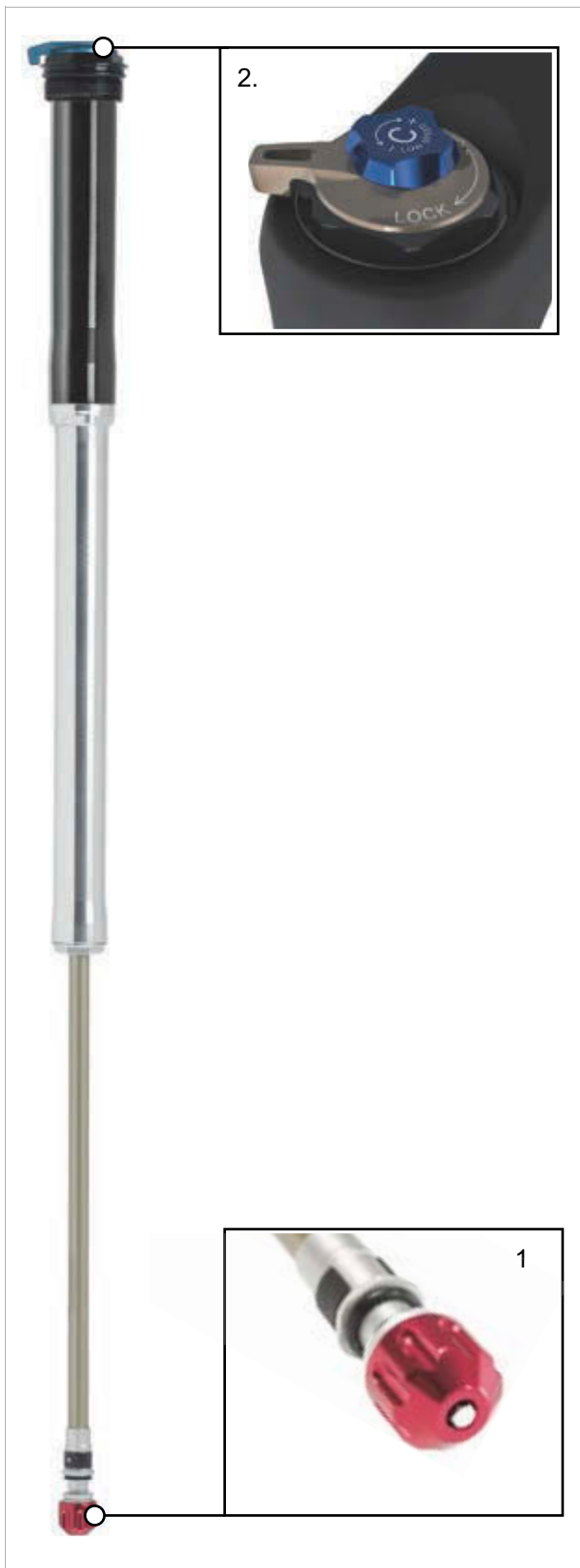
Figure 29: HLO operating elements
