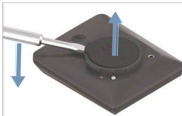
Figure 150: Prying open the battery compartment lid
