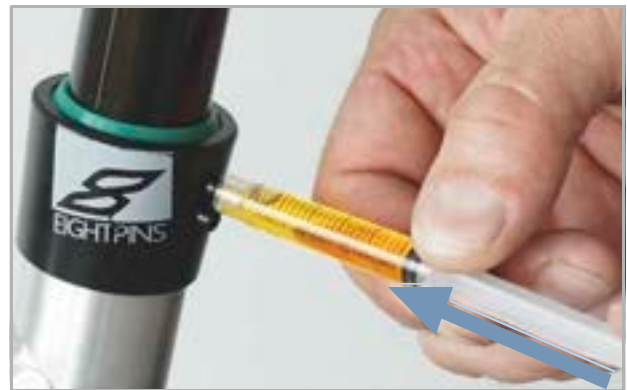
Figure 192: Lubricating the Eightpins seat post
