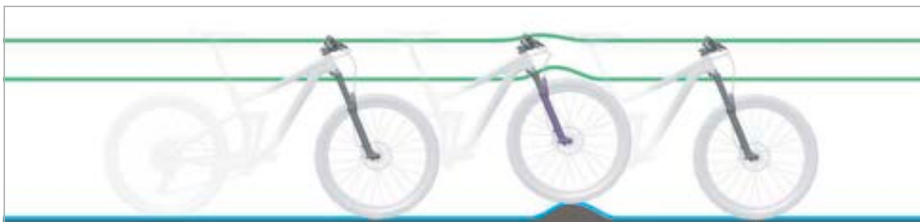
Figure 136: Optimum fork ride performance over bumps
