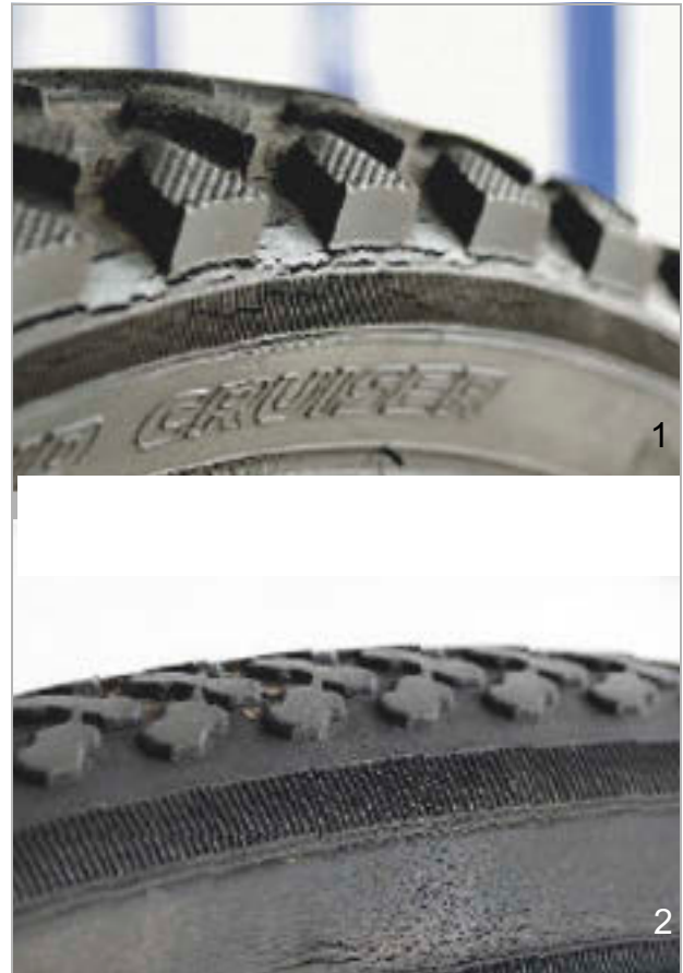
Figure 195: Examples of fatigue cracks (1) and ageing cracks (2)
