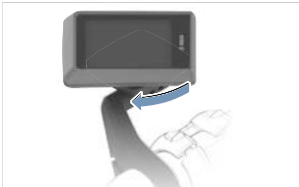
Figure 153: Turning the display clockwise
