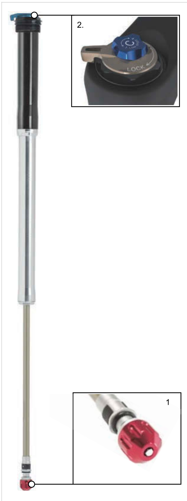
Figure 27: LO operating elements
