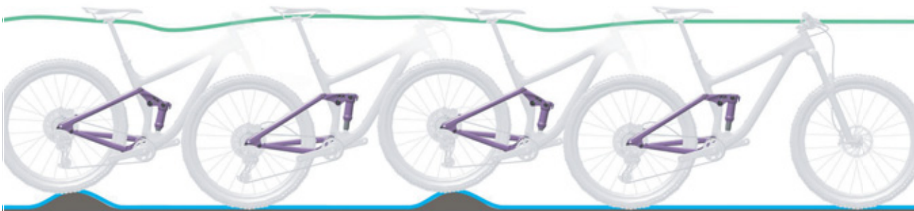
Figure 62: Optimum rear frame damper riding performance
