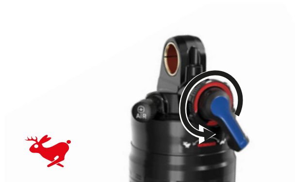
Figure 67: Increasing the rebound speed
