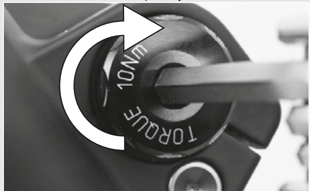
Figure 26: Tightening the inserted axle
