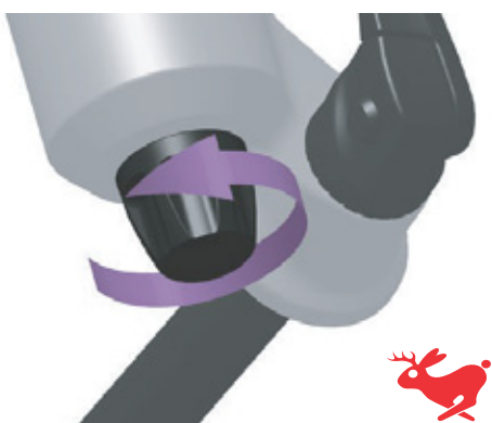
Figure 92: Turning rebound damper towards hare symbol
