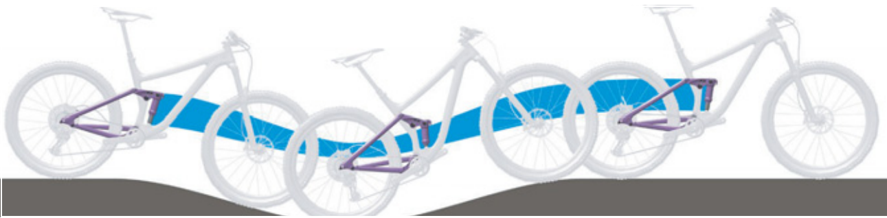
Figure 101: Excessively soft suspension in the rear frame damper on hilly terrain
