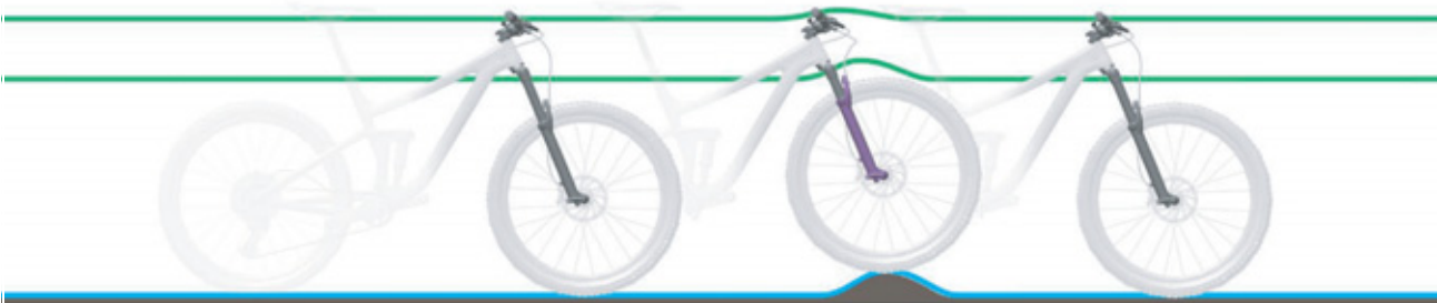
Figure 76: Optimum performance over bumps
