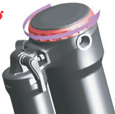
Figure 100: Turning rebound damper towards hare symbol
