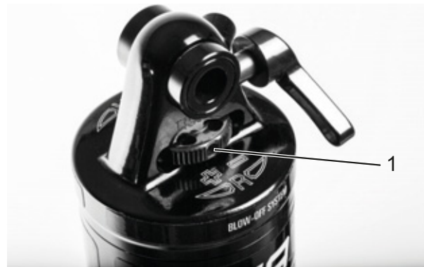
Figure 64: Suntour rebound adjuster wheel (1) on the rear frame damper
