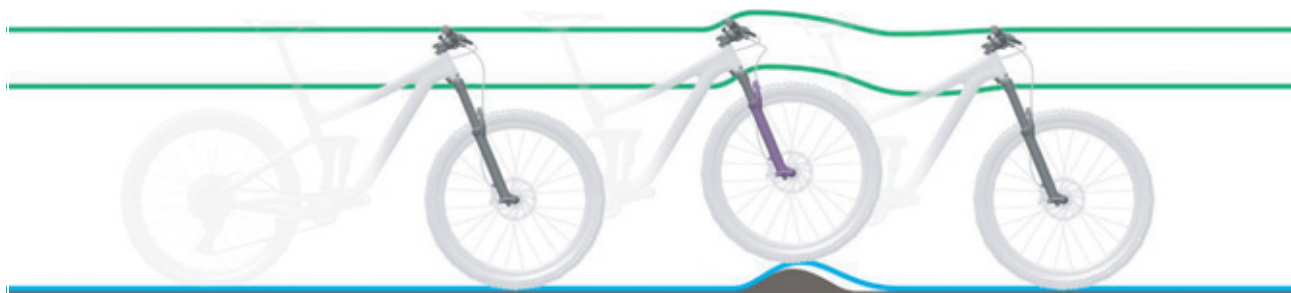
Figure 95: Excessively hard damping in the suspension fork on bumps
