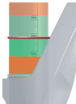
Figure 58: Mandatory sag range (green) and forbidden sag range
