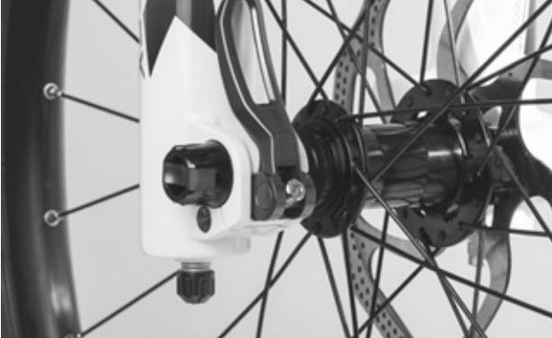
Figure 84: Adjusting the quick release clamping force
