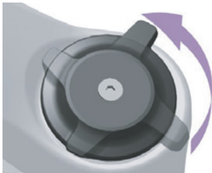
Figure 79: Changing compression adjuster to a softer setting
