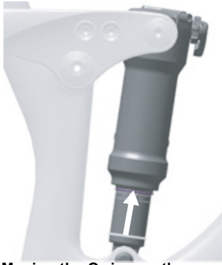
Figure 60: Moving the O-ring on the rear frame damper
