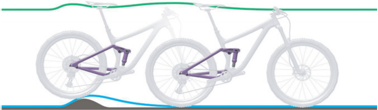
Figure 103: Excessively hard damping in the rear frame damper on bumps
