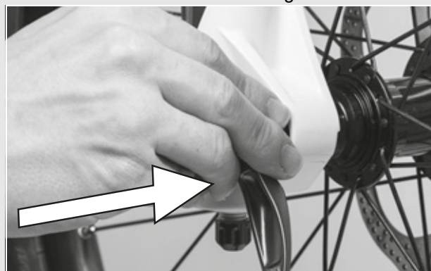
Figure 43: Pushing the quick release in
