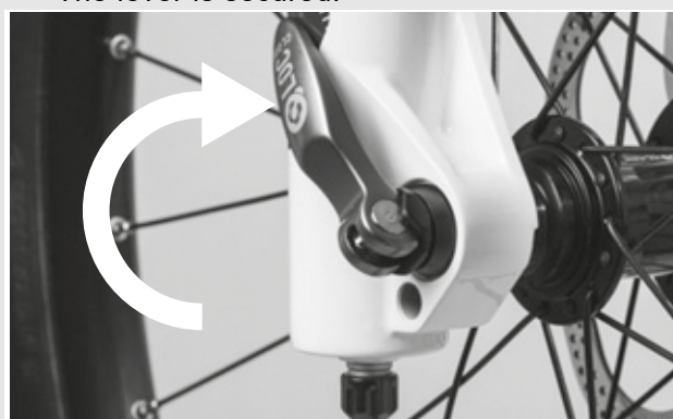
Figure 45: Closing the quick release
