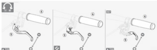
Figure 59: Setting the grip distance on a Magura disc brake lever
