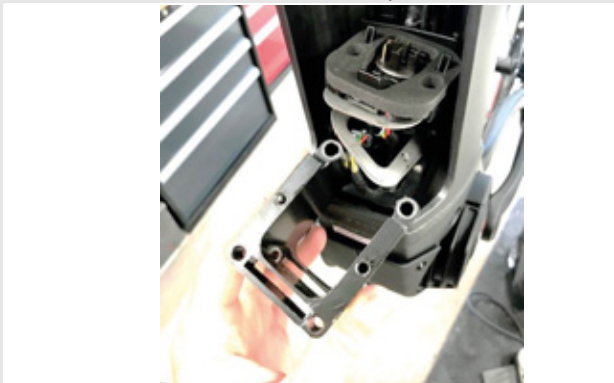
Figure 27: Pulling out the PowerTube adapter
