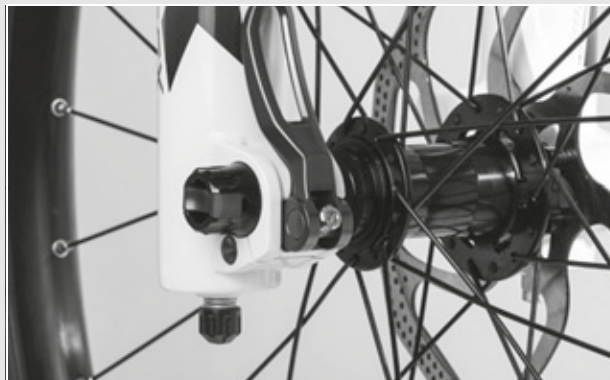
Figure 40: Perfect position for the clamping lever
