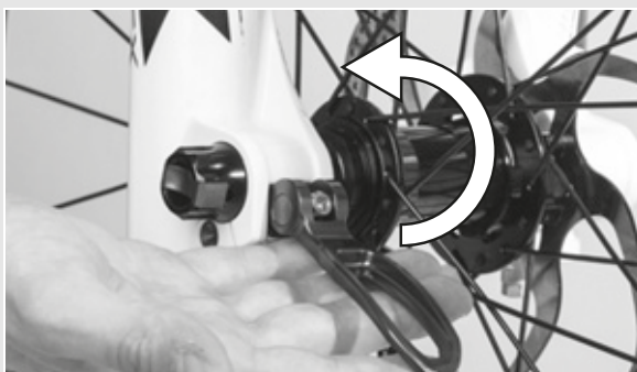
Figure 39: Securing the lever
