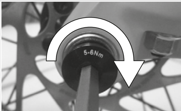
Figure 33: Tightening the securing screw
