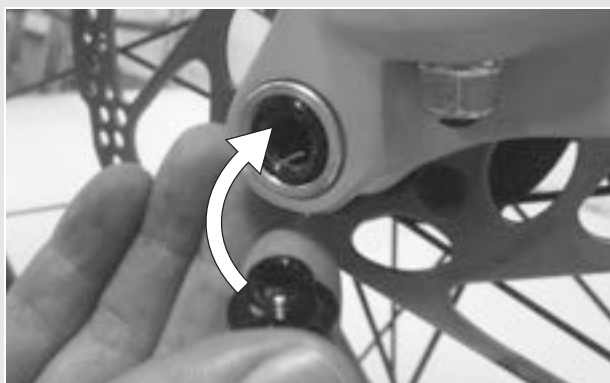
Figure 32: Pushing the quick release lever into the axle
