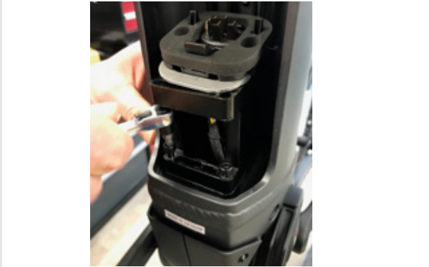
Figure 25: Removing the 4 mm hexagon screws
