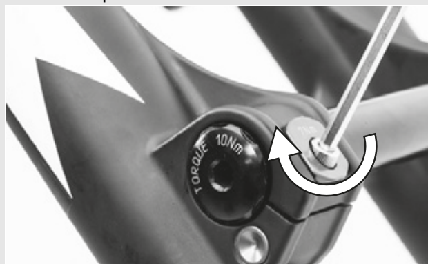
Figure 35: Tightening the securing clip
