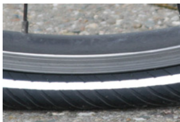
Illustration 93 : Pression largement insuffisante
