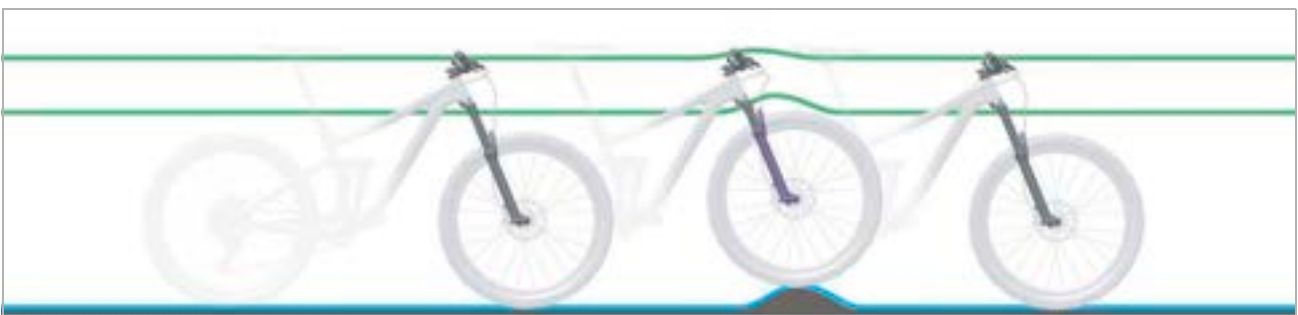
Figure 15: Optimum fork ride performance over bumps
