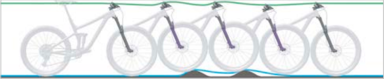
Figure 189: Suspension fork rebounding too slowly
