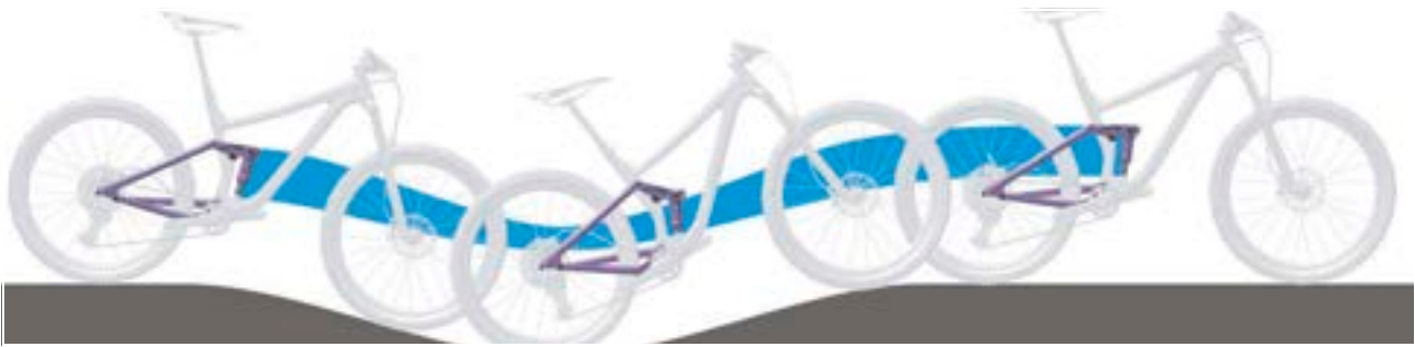
Figure 197: Excessively soft suspension in the rear frame damper on hilly terrain
