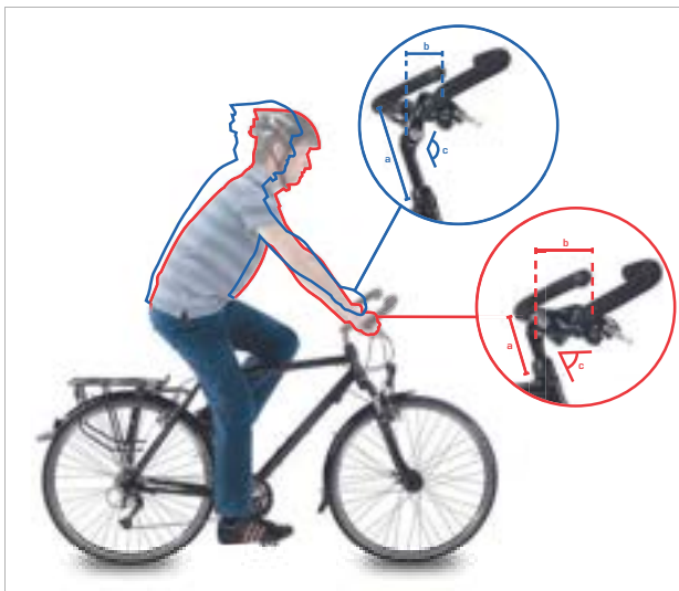
Figure 103: City bike (blue) and trekking bike position (red) by changing the angle
