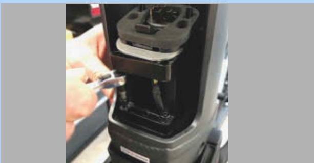
Figure 64: Removing the 4 mm hexagon screws
