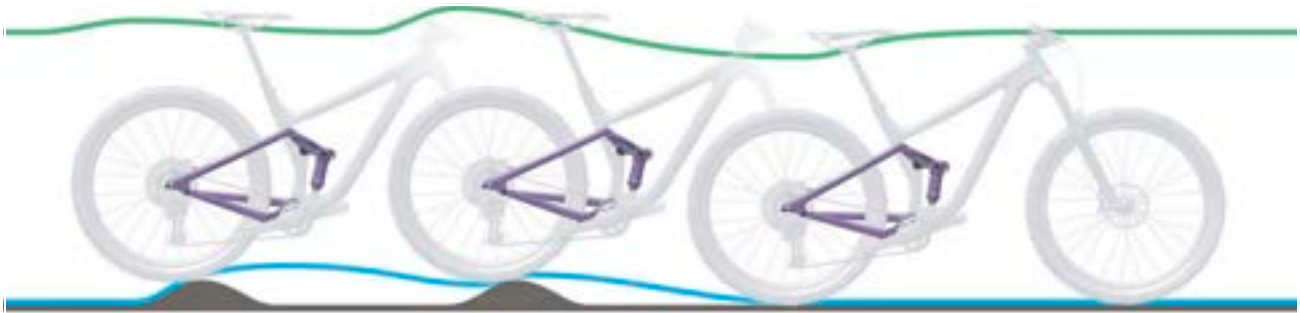
Figure 195: Rear frame damper rebounding too slowly
