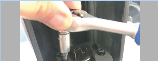
Figure 63: Undoing screws on battery mount
