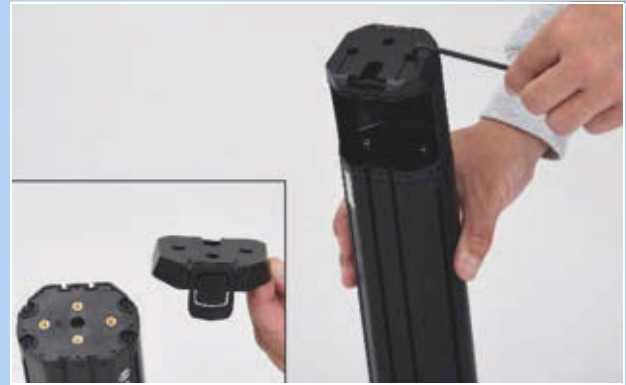
Figure 74: Fastening the battery mounting plate
