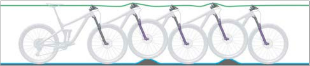
Figure 16: Optimum fork ride performance
