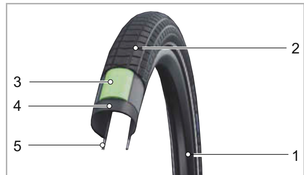
Figure 24: Structure of tube-type tyre
