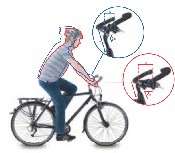
Figure 124: City bike (blue) and trekking bike position (red) by changing the angle
