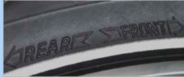
Figure 68: Rotation direction arrow on MTB tyres
