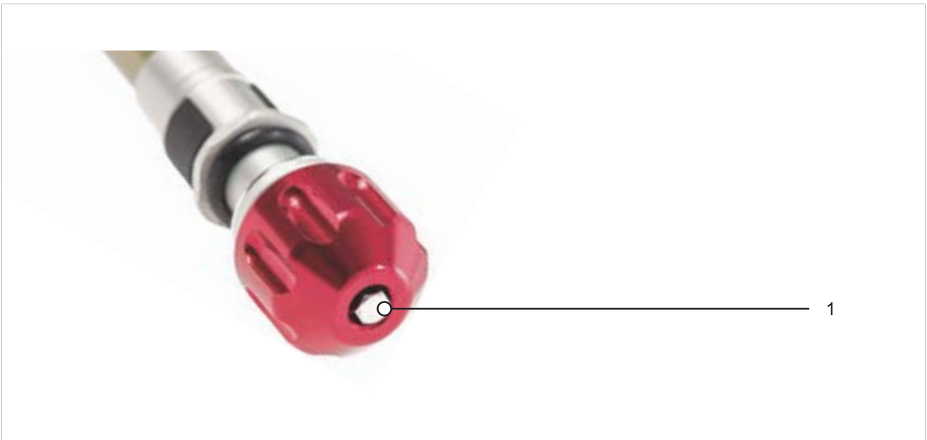
Figure 175: Example of SR SUNTOUR rebound screw (1)
