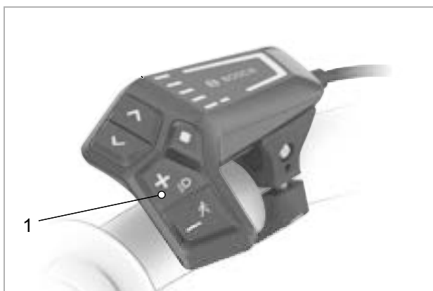
Figure 124: Position of riding light button (1)
