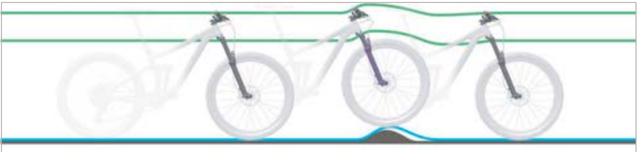
Figure 177: Excessively hard damping in the suspension fork on bumps
