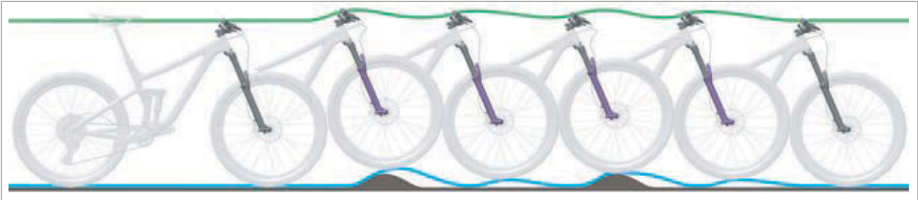
Figure 172: Suspension fork rebounding too quickly
