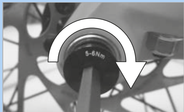
Figure 56: Tightening the securing screw
