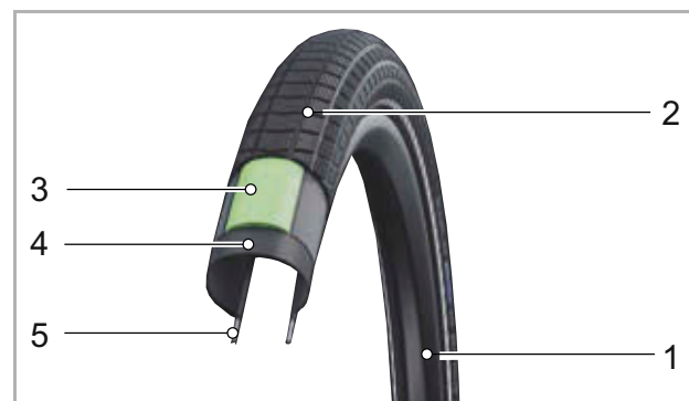
Figure 21: Structure of tube-type tyre
