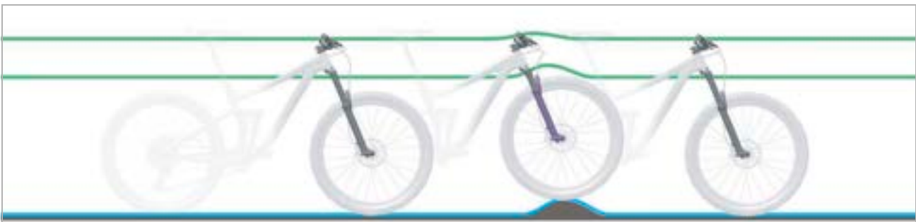
Figure 106: Optimum fork ride performance over bumps
