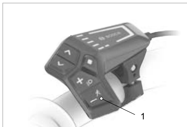
Figure 126: Position of push assist button (1)
