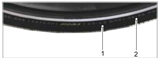
Figure 137: Tyre pressure specification in bar (1) and psi (2)
