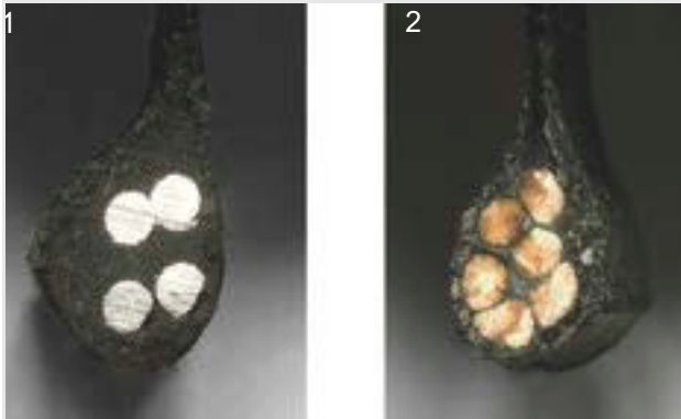
Figure 22: Steel bead core (1) and Kevlar bead core (2)
