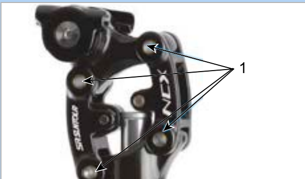
Figure 170: SR SUNTOUR suspension seat post lubrication points
