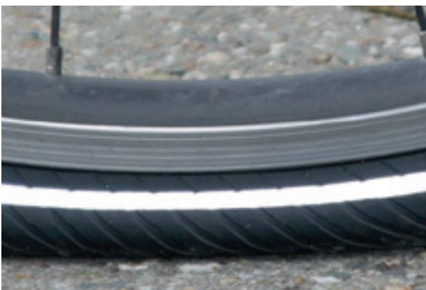
Illustration 127 : Pression largement insuffisante
