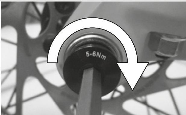
Figure 27: Tightening the securing screw
