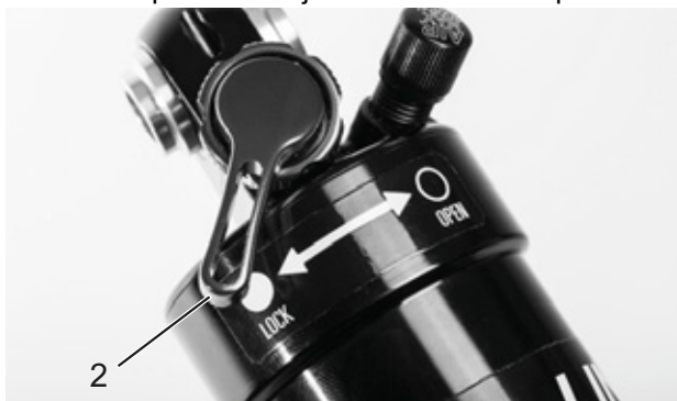
Figure 81: Suntour compression adjuster closed (2)
