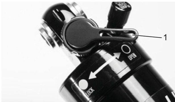
Figure 80: Suntour compression adjuster open (1)
