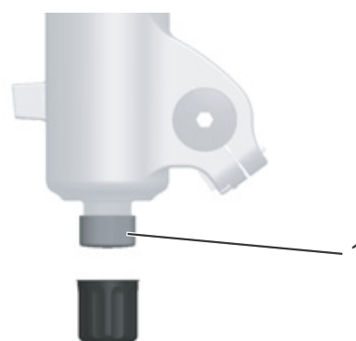
Figure 63: FOX rebound adjuster (1) on the fork
