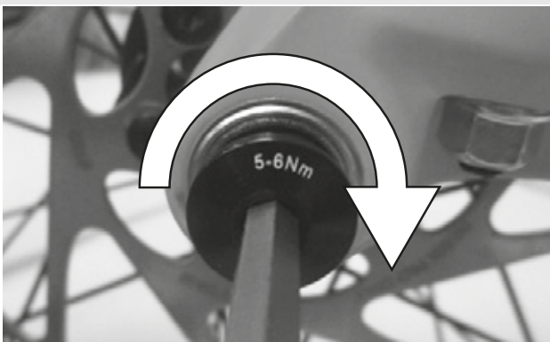
Figure 31: Tightening the securing screw
