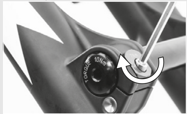
Figure 33: Tightening the axle
