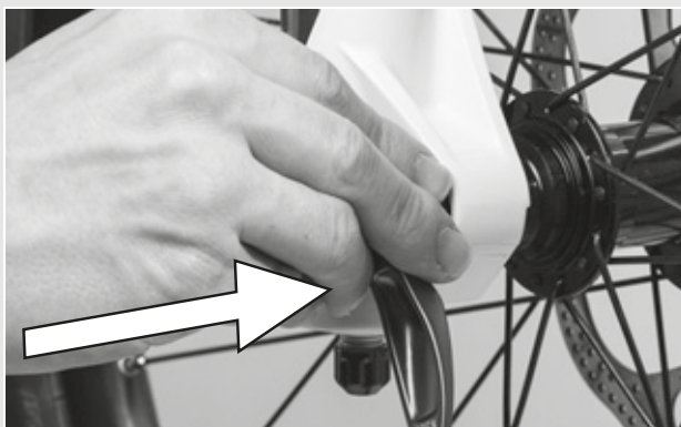
Figure 41: Pushing the quick release in
