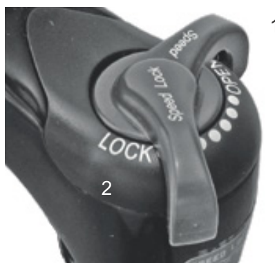
Figure 79: Suntour compression adjuster with the OPEN (1) and LOCK (2) positions
