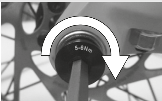
Figure 28: Tightening the securing screw
