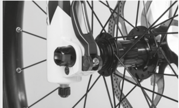
Figure 84: Adjusting the quick release clamping force
