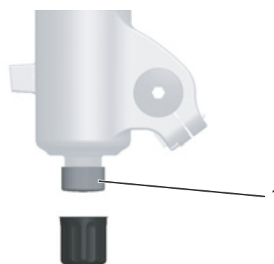
Figure 60: FOX rebound adjuster (1) on the fork
