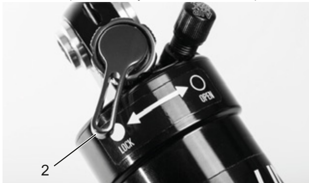
Figure 78: Suntour compression adjuster closed (2)
