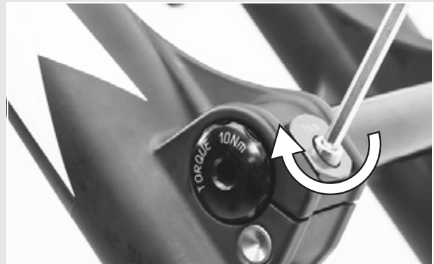
Figure 30: Tightening the axle
