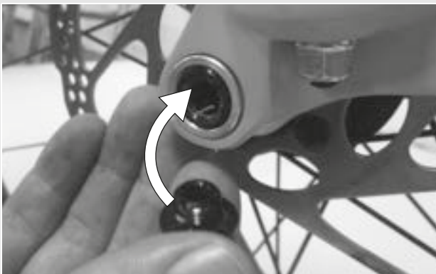
Figure 27: Pushing the quick release lever into the axle
