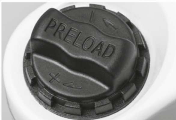
Figure 43: Negative deflection setting wheel on the suspension fork crown
