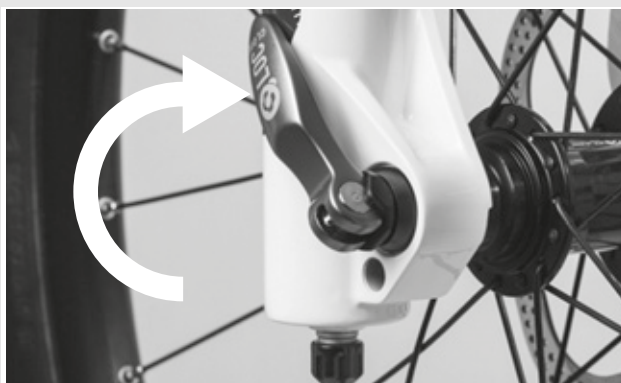
Figure 26: Closing the quick release
