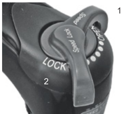
Figure 49: Suntour compression adjuster with OPEN (1) and LOCK (2) positions
