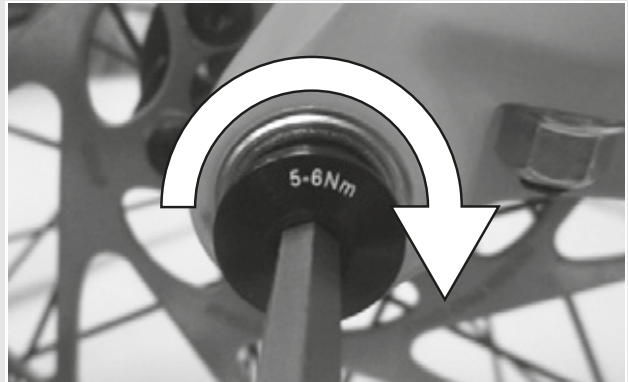
Figure 14: Tightening the securing screw
