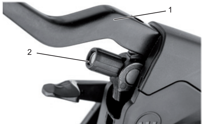
Figure 67: Brake lever (1) of the hydraulically operated rim brake with setting bolt (2)
