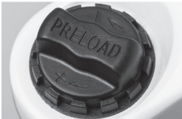
Figure 47: Negative deflection setting wheel on the suspension fork crown
