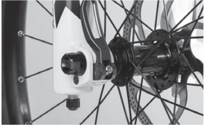
Adjusting the quick release clamping force
